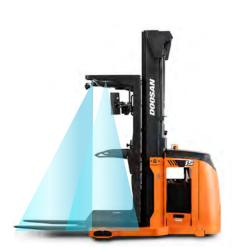
**Bright LED Platform Lights** Operator compartment lighting provides better visibility even in dark operations.
