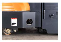
Maintenance Friendly Grease zerks at all pivot points make servicing easy and convenient, increasing up-time
