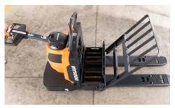
**Battery Roller System is Standard** Saves time and effort during battery change-outs
