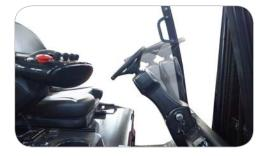
Adjustable Steering Column The operator can adjust the position of the column for convenience and comfort
